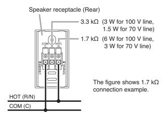
The input power is set to 6 W (100 V line) by connecting the Hot line to the N-terminal, and 3 W (100 V line) by connecting it to the R-terminal.
