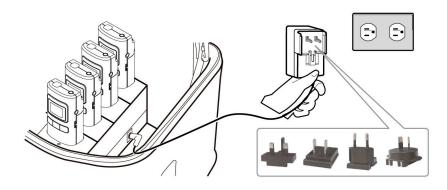
1-2 Insert the transmitter or receiver into the compartment in accordance with direction as shown in the picture below.
