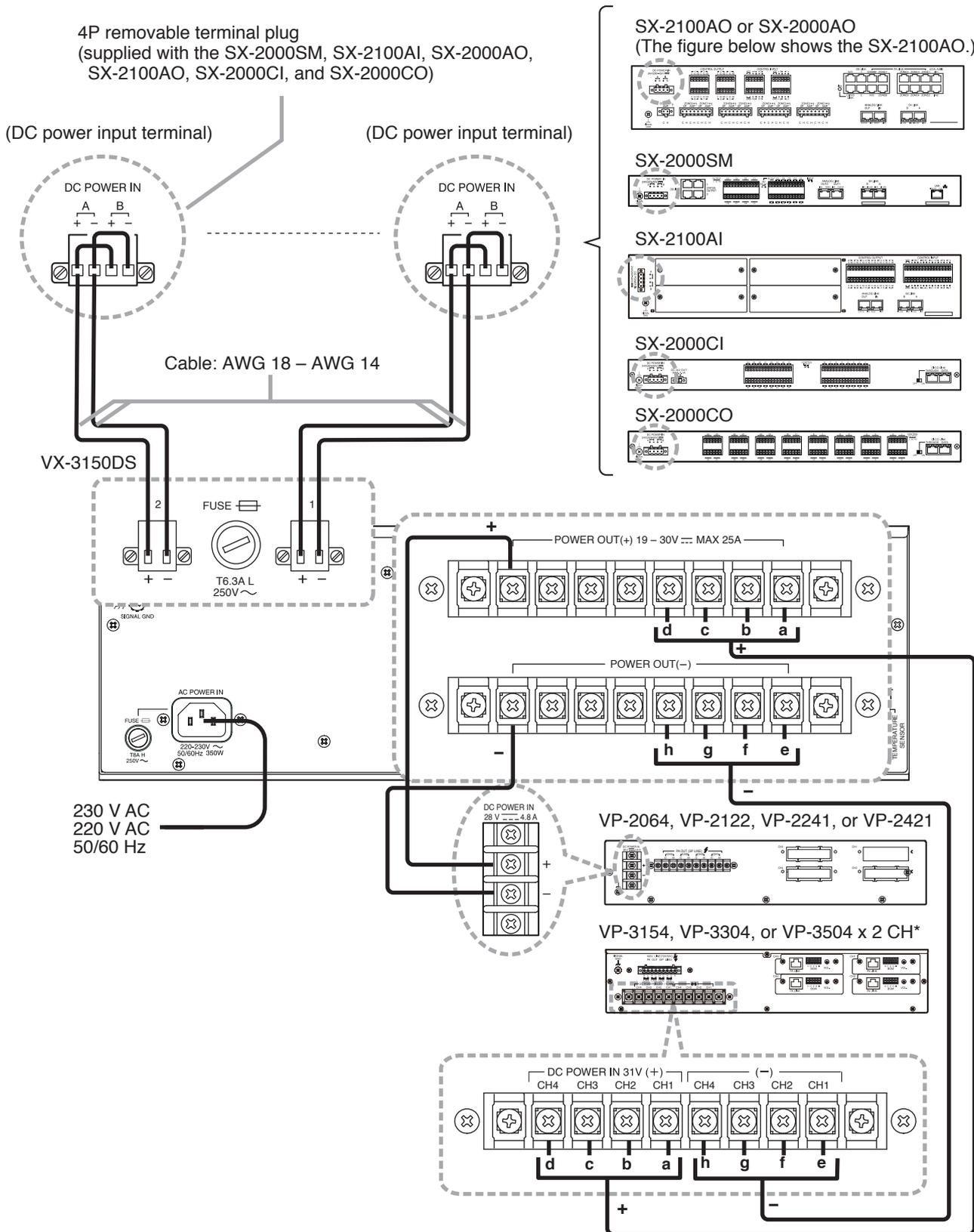
\* VP-3504 x 2 CH: That only 2 channels can be used when VP-3504 connect to VX-3150DS.
