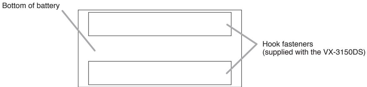
When replacing the batteries, 4 each of fastener hooks and loops, and a thermal insulating sheet listed below are also required. Consult your nearest TOA dealer on how you can obtain them.
