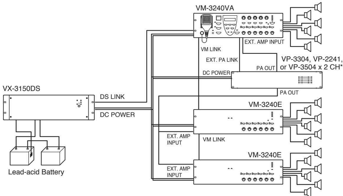
\* VP-3504 x 2 CH: That only 2 channels can be used when VP-3504 connect to VX-3150DS.
