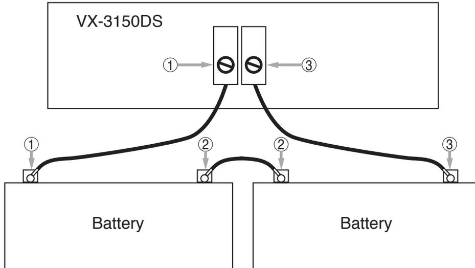
Touch the battery contacts and the screw tops of the battery connector of the VX-3150DS with the measuring tips as shown above.
