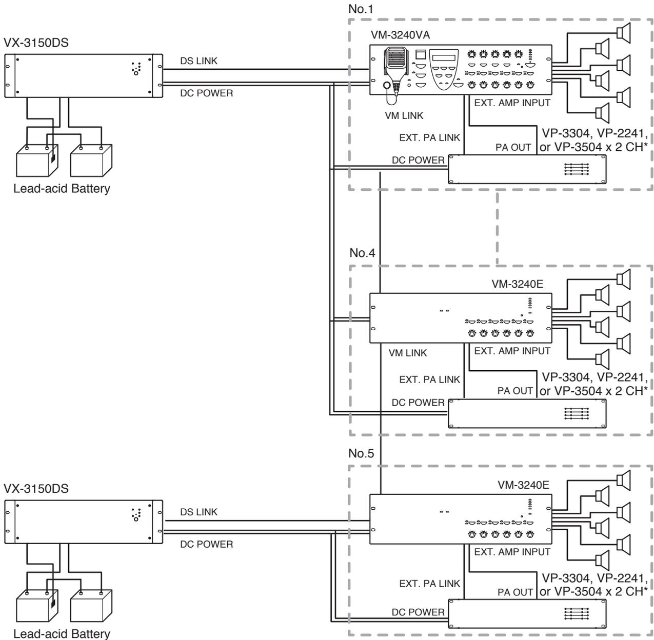
\* VP-3504 x 2CH: That only 2 channels can be used when VP-3504 connect to VX-3150DS.
