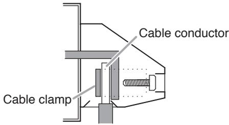
**Incorrect position of the cable insertion**
