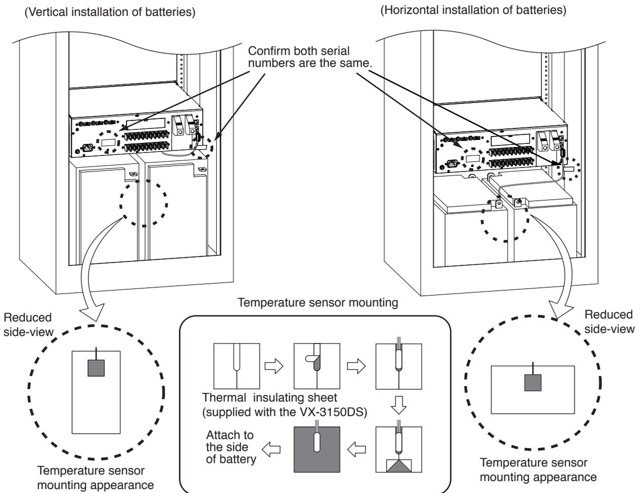
**Step 1.** Clean the exterior surface of the battery using a soft damp cloth.
