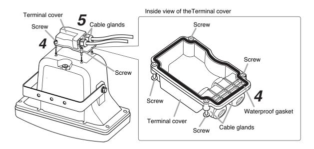
Step 7. Securely tighten the cable glands.
