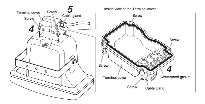
Step 5. Securely tighten the cable gland.
