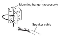
**Step 4.** Connect the speaker cable to the screw terminal.
