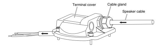
Step 3. Connect the speaker cable according to the polarity indication at the screw terminal.
