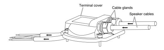
**Step 5.** Connect the speaker cables with the same polarity to each terminal according to the polarity indication at the screw terminal.
