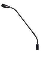
The TS-923 Microphone is a dedicated component of the Infrared Conference System's Chairman unit and Delegate unit. Its mic head is equipped with an illuminated display ring that allows the status of the units in use to be monitored at a glance. Its gooseneck has two flexible parts, making it possible to adjust the microphone to an optimal position for the user.
