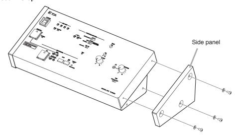
**Step 2.** Attach the MB-TS920 Rack mounting bracket to both sides of the Central unit. Use the screws removed in **Step 1.**
