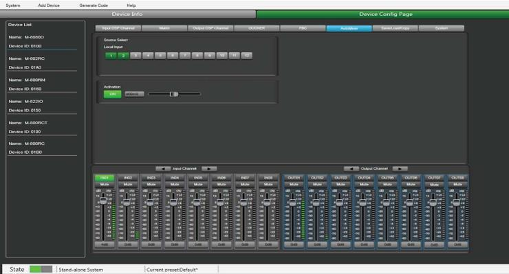
Add the local input CH 1 and CH2 open setting to the automatic mixing function. Input the audio source from two channels. Click the ON button of Active Time and push the fader to set the start mixing time of the CH 1 and CH2 signal. For example, drag the fader to 900ms, the sound source of channel 1 will be at 900ms, and the mixing function is added.
