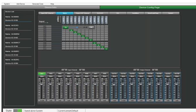
This part of the software is used to route inputs through a graphical representation as a matrix. By clicking on the gray boxes several inputs can be assigned to several outputs. If the connection is active the box turns green, otherwise it remains gray.
