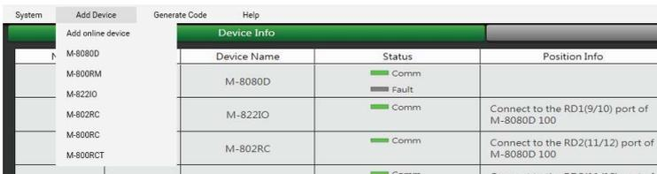
There are 7 kinds of machine in the Matrix system. You can select any device to input ID to view this device parameter (like Demo ).
