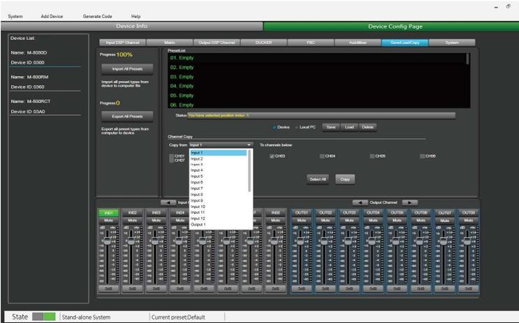
Select the input channel Input 1 to copy to CH03. Click the COPY button, the parameters of input channel 1 will be copied to CH03.
