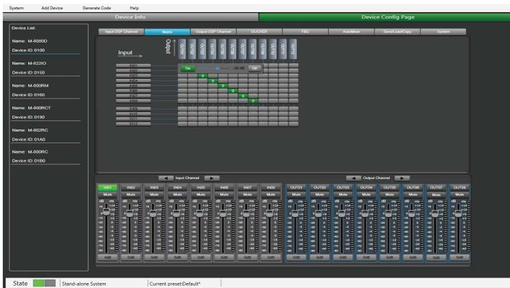
Assign input 1 to output 1, when the sound is adjusted to -29dB, press OK. The sound of channel 1 will be adjusted to -29dB.
