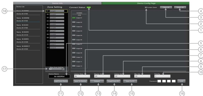
This function is a partition setting, with audio routing function, can control up to 12 partitions. Distribute audio to different partitions, and easily manage partitions by adjusting the sending time / volume / priority.
