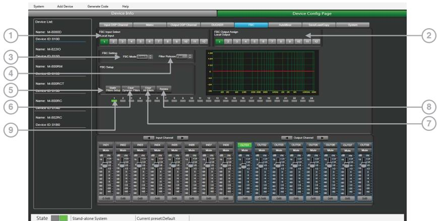
FBC (Feedback compression) function can effectively suppress howling expansion volume, ensure voice transmission quality, high fidelity, and clear sound.
