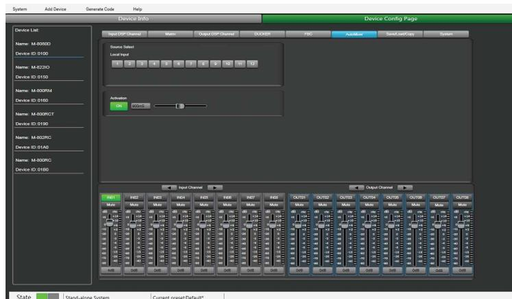
The Auto mixer automatically controls the gains of multiple microphones in real time, dramatically reducing feedback, noise and comb-filtering from adjacent microphones. It maintains a consistent system gain, even when multiple speakers are talking simultaneously, and makes perfectly matched crossfades, without any signal compression.
