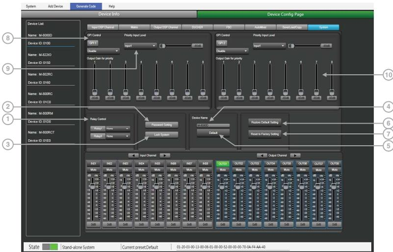
1. **Relay Control:** It is used to control external devices. Allow end users to control their actions.
