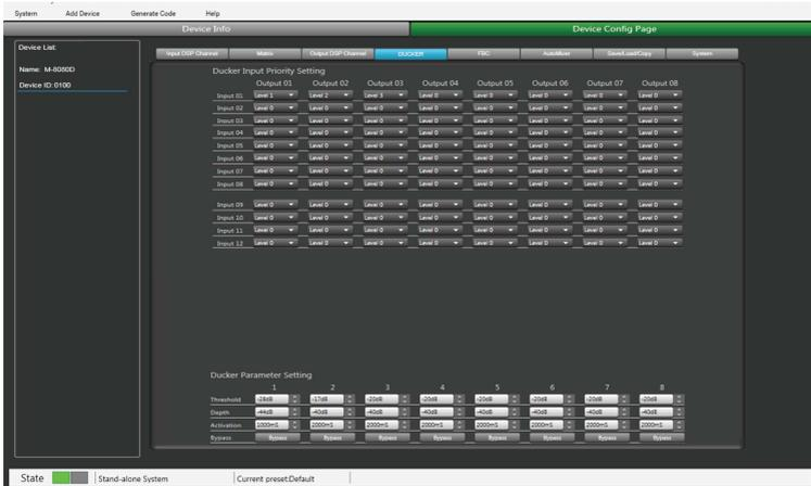
The current setting sets channel 1 to level 1, channel 2 to level 2, and channel 3 to level 3. At the same time, the Threshold, depth, and Active time are set at the bottom of the page. The audio source will be output according to the previously set priority and other parameters.
