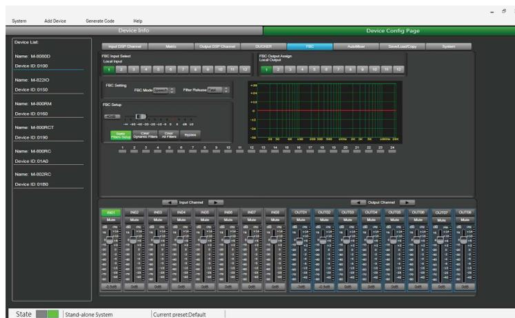
Turn on local input / output 1. The corresponding input signal is sent to the FBC module for processing, and the corresponding button is lit to output the signal after FBC processing to the corresponding output channel. Click "Static Filter Setting" to enter the static filter setting mode.
