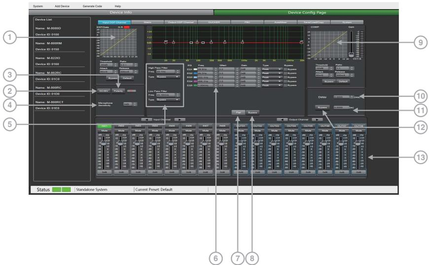
**1. EXP/Gate:** The gate attenuates signals below the threshold value, and allows signals above the threshold value to pass. When the signal is beyond the threshold, the output signal remains identical to the input signal. By adjusting the value of the ratio to its maximum, the Expander is transformed into a Noise Gate.
