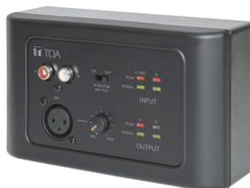
The **M-822IO** is a remote audio input and output module providing 2 x analog channels IN and 2 x analog channels OUT. The device includes built-in A/D and D/A converters processing digital audio AES3 signals from and to the **M-8080D**.
