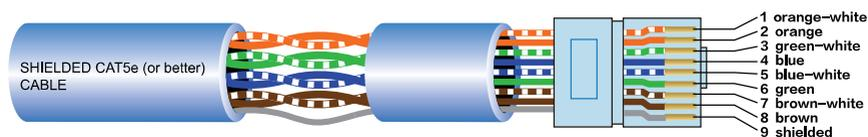
The green pair is reserved for data communications between **M-8080D** and remote device. Data communication is needed to send configuration information, software update and status information from **M-8080D** to remote device.
