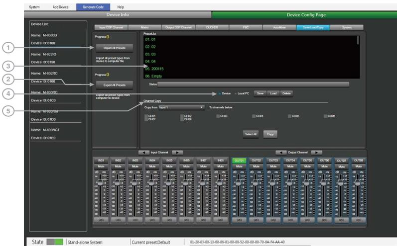
This menu is used to manage the backup parameters. These data can be stored directly in the internal memory of host as a preset. Its memory contains a total of 16 presets.
