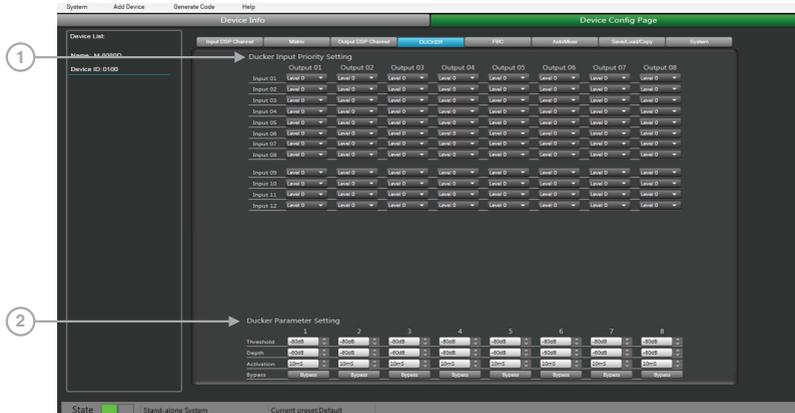
The principle of the Ducker is to attenuate one or several channels when priority signals are activated. The main applications are automatic speech for conference or priority messages. E.g. Use the host microphone signal to control the background music volume. The host automatically reduces the background music volume when speaking. After the speech, the volume of BGM music is automatically restored.
