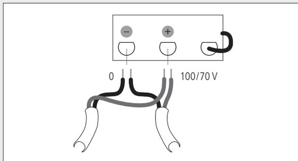
Connections with the audio line are made by using the internal ceramic terminal strip (it is necessary to remove the rear cover by loosening its three screws).
