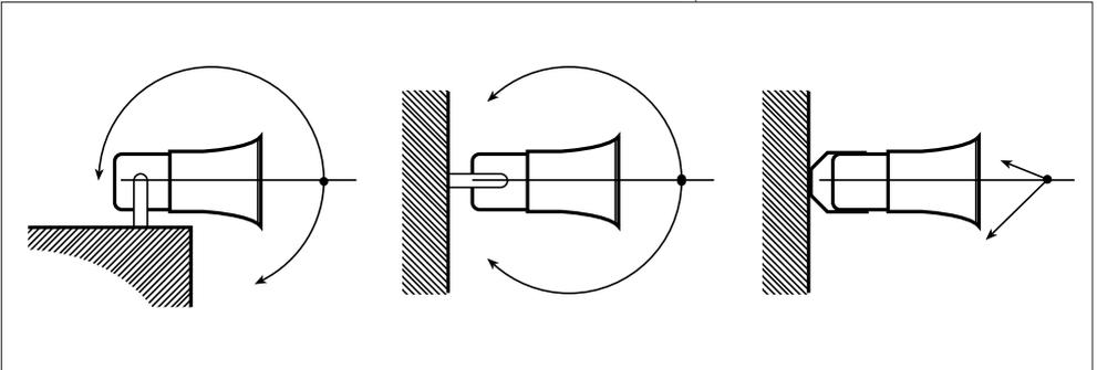
Aim the loudspeaker to the listening area and fix its position by tightening the two bolts of its mounting bracket.
